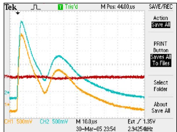
Fig. 6 – RSO twin signals as picked from a rotor winding without shorted turns. The quasi-straight line is the sum of the signals with one of them inverted
