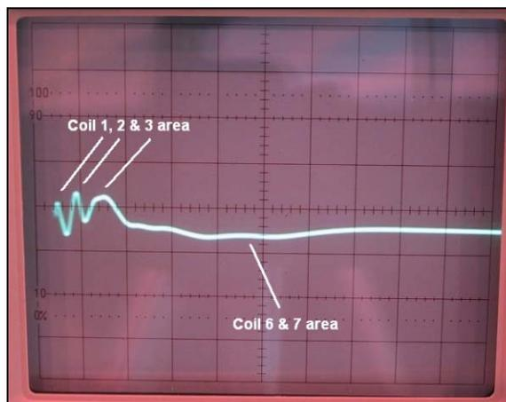
Fig. 8 RSO trace showing multiple shorted-turns
