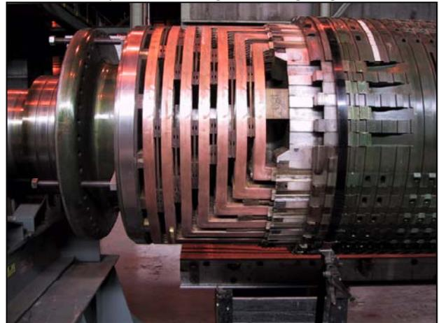
Fig. 1 Typical field endwinding
