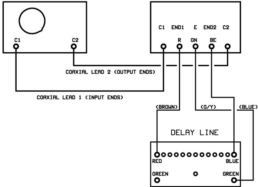
Figure 0.2.1 Connection diagram using delay line
