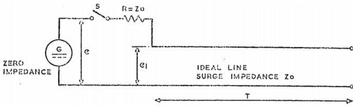
FIG. 3. RECURRENT SURGE GENERATOR AS A REFLECTOMETER
