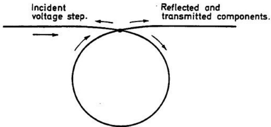
**Figure 1.11 Simple representation of a shorted turn**
