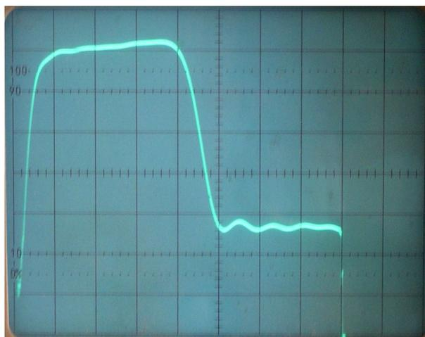
**Figure 0.6.2 (a) Input ends waveforms with  $R_1 = 100$  Ohms and  $R_2 = 0$  Ohms**
