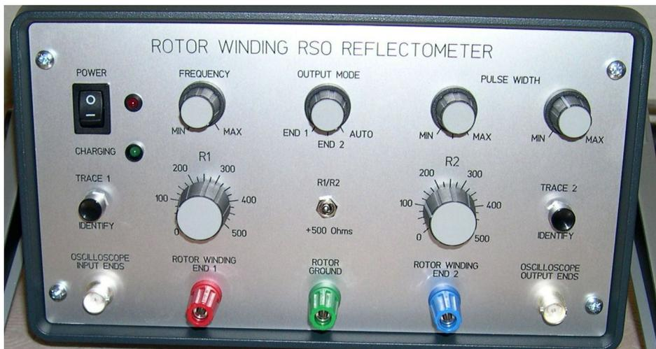
The **TDR100RB** is similar in operation to the **TDR100**. The main difference is that the **TDR100RB** contains a maintenance-free 12 volt 2.0 AH rechargeable NiMH battery pack, giving over 15 hours continuous use under average operating conditions. There is also an additional switch on the front panel to turn on the instrument for both battery and mains operation. Note that the equipment can be used while the battery is being recharged.
