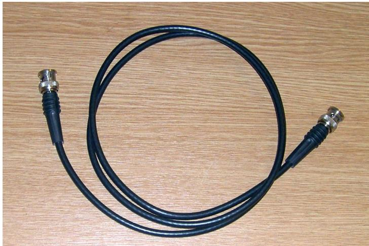
**Figure 2.5. Oscilloscope Lead**
