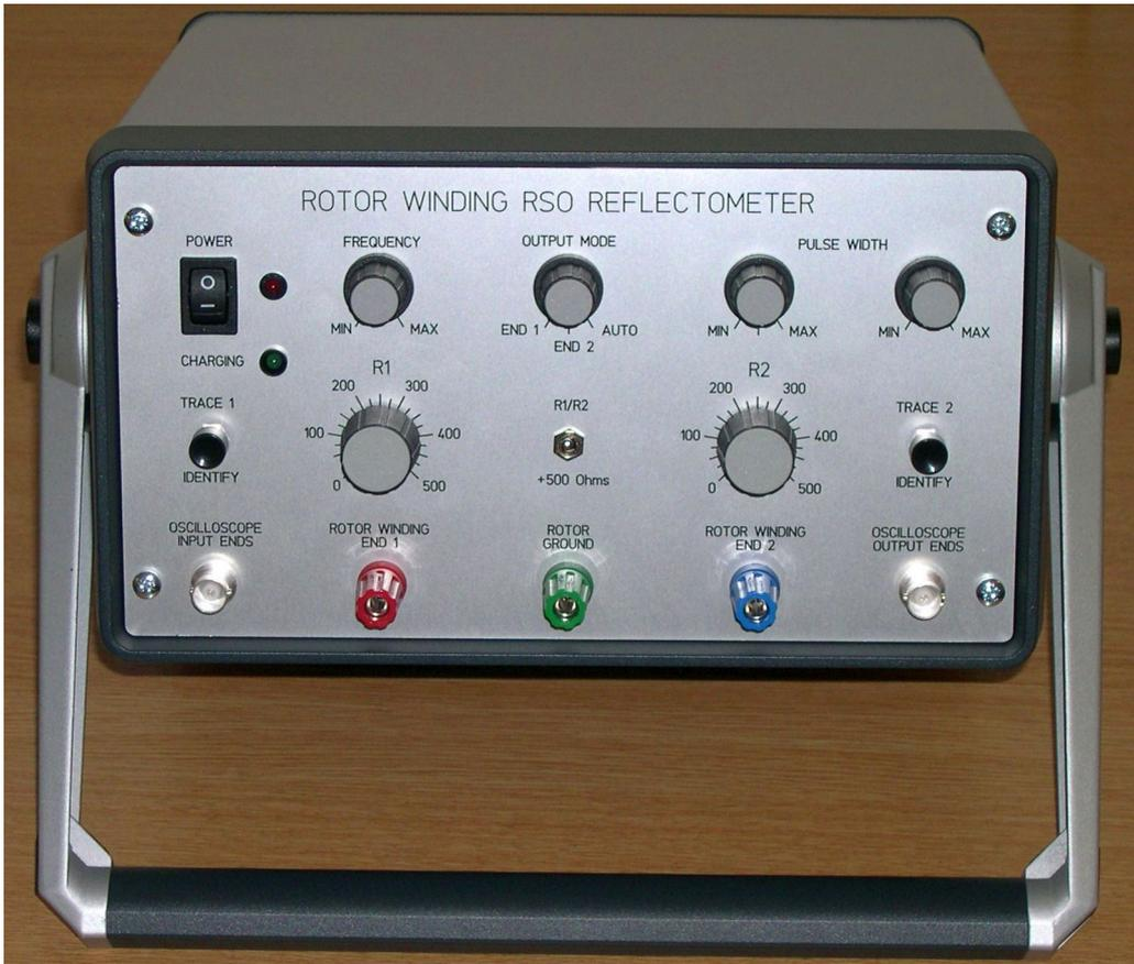
**FRONT VIEW OF TRDR100RB ROTOR REFLECTOMETER**
