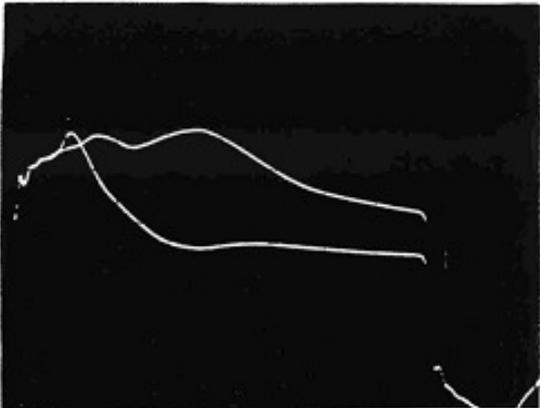
(a) Short circuit to rotor body at end of 5th slot coil (16 coils in winding)
