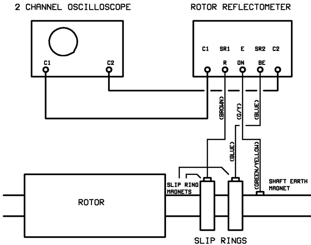
Note that the colours in parentheses eg (BROWN) refer to the connecting leads, while the abbreviated colours eg R (RED) etc. refer to the 4mm banana plugs and terminals.
