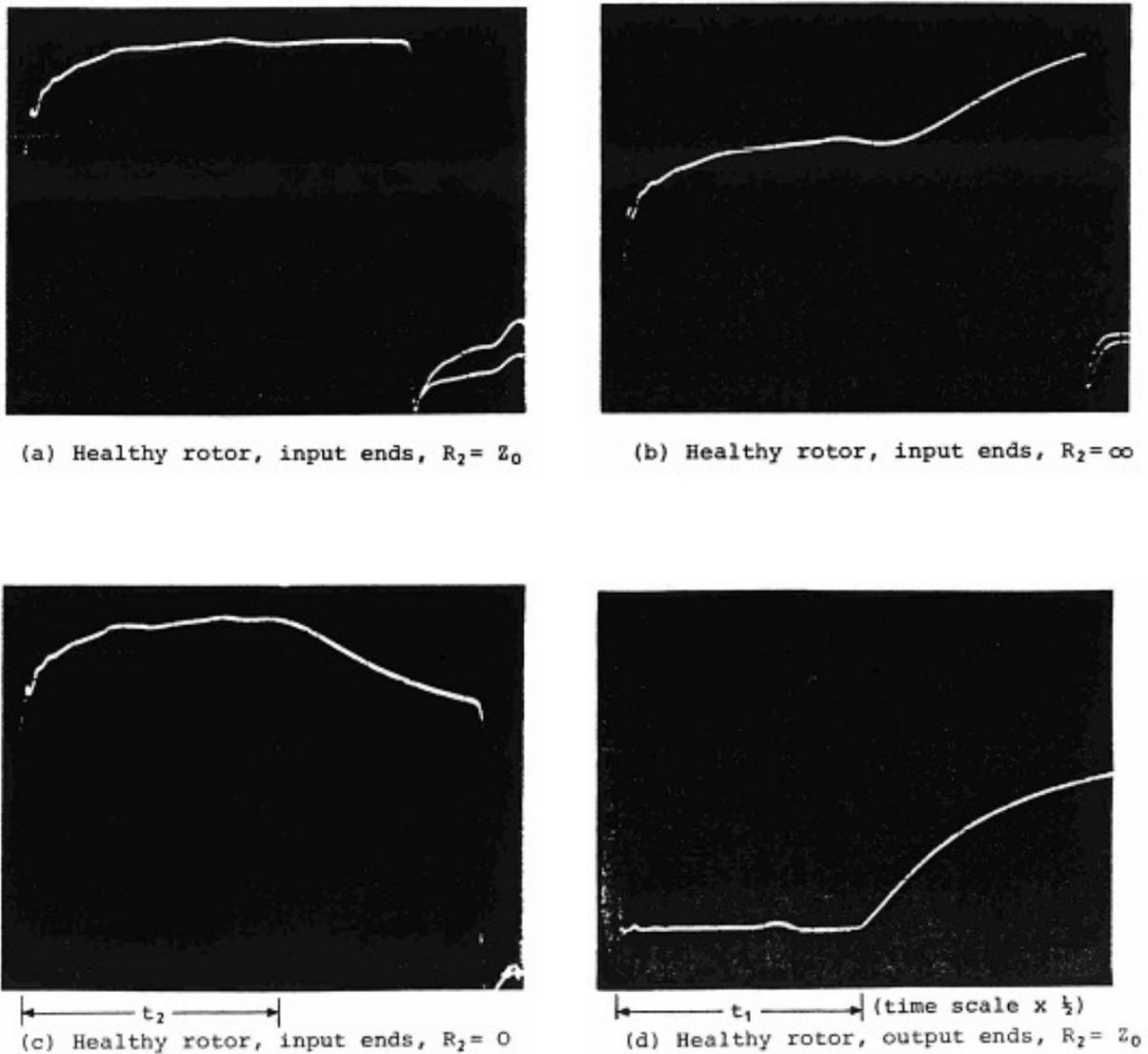
**Figure 3.1. Typical waveforms for a fault-free rotor winding**
