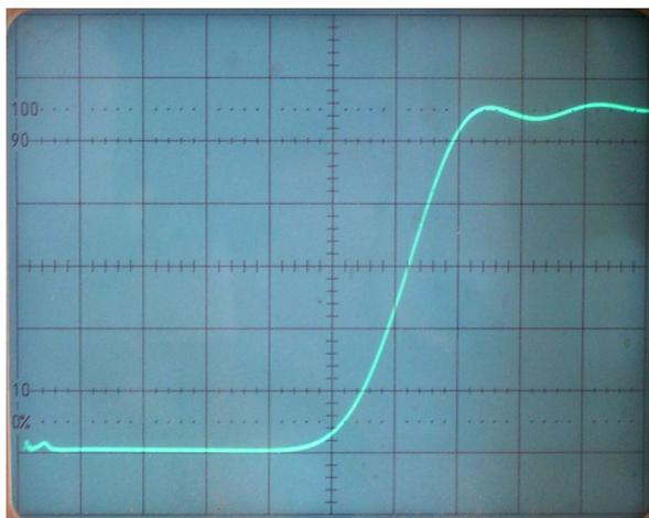
**Figure 0.5.1 (b) Output ends waveforms with  $R_1$  and  $R_2 = 100$  Ohms**
