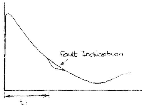
Smith-Moat trace for the typical 500MVA generator rotor used in Appendix 1
