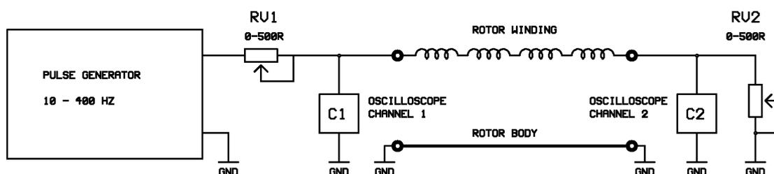
**Figure 1.4 Rotor winding test method**
