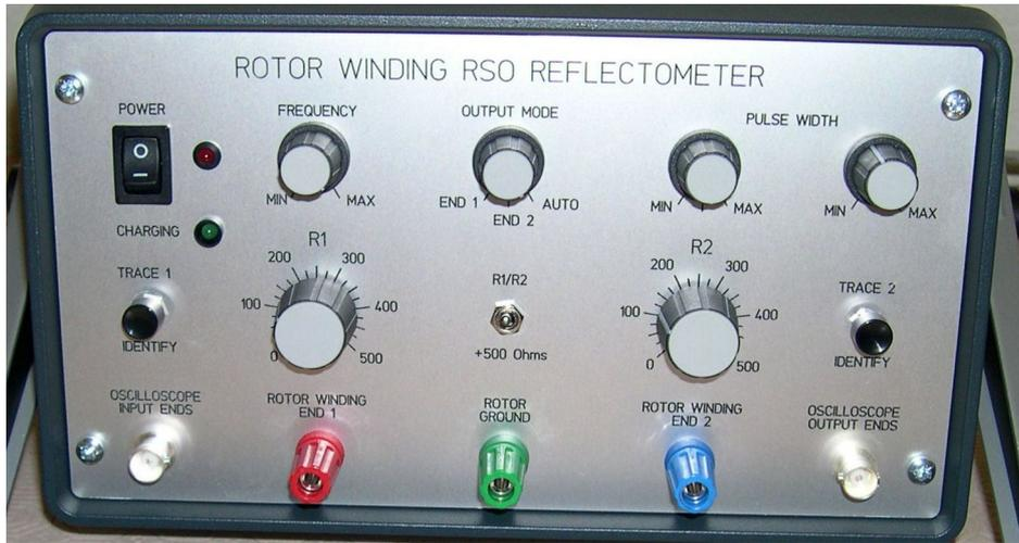
**Figure 2.4 Reflectometer front panel controls (TDR100RB)**
