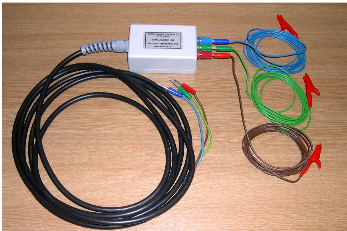
Figure 2.2 Rotor test leads and connection module
