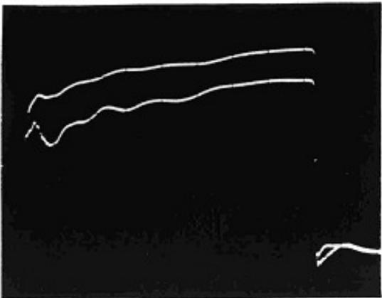
(c) High resistance joint ( $32\Omega$ ) near one end of winding.
