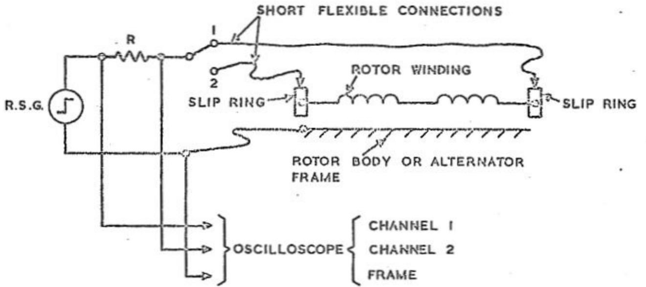
FIG. 2. CONNECTION OF R.S.G. TO ROTOR WINDING
