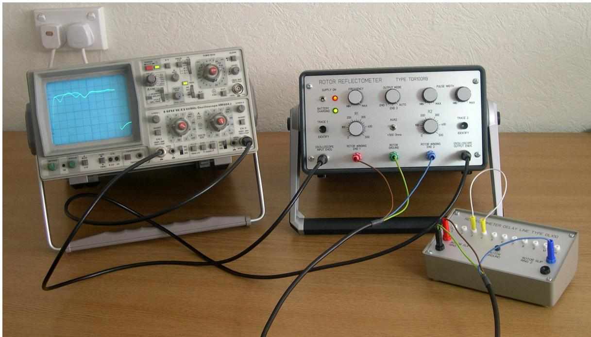
**Figure 4.3 Use of Delay line test unit \***
