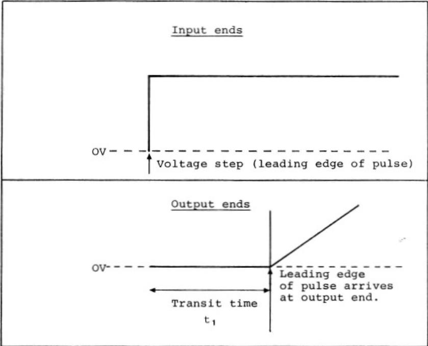
**Figure 1.7 Simplified oscilloscope traces for fault-free rotor winding**
